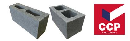
Dense concrete blocks with solid, hollow and cellular cores. Dense Blocks are produced using responsibly sourced and sustainable high-quality sands and aggregates. Available in a close textured/paint grade finish. Suitable for ground conditions up to DS3. Compliance with EN1996-1 Group 1 Manufacturing Standard BS EN 771-3:2011
